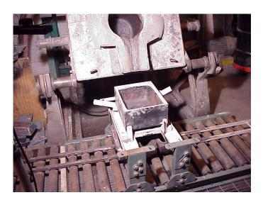
One of my projects, next to the 400lb induction furnace used for all ferrous melting. This was for the casting of stainless steel. I welded stuff together, like the frame on the roller table to take ingot moulds, joined two roller-tables, fabricated the frame for the tundish,  $\dots$  I also formed and fired the refractory.
