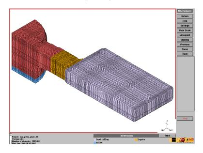
A fully-sound 3/4 inch thick casting (predicted). This outcome is obtained because the casting is less thick (0.75inch) than the ingate is high (0.9inch) and there is oil-heating of the ingate area / water-cooling of the die.
