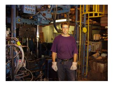
Me by a vertical squeeze-caster - an Ube 350T model used to cast Aluminium. I was involved in refining the conditions used with this machine, in order to get fully-sound castings at large sizes.
